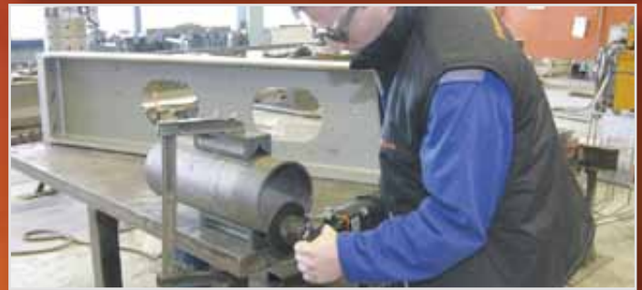
Initial bores from Ø 20 mm.
