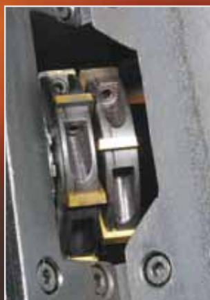
2 milling disks coupled with 6 indexable inserts each
