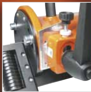
Fine Adjustment of Milling Depth/Bevel Width
