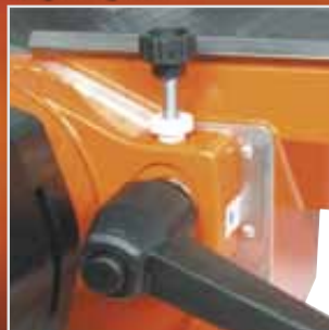
Fine Adjustment of Milling Depth/Bevel Width
